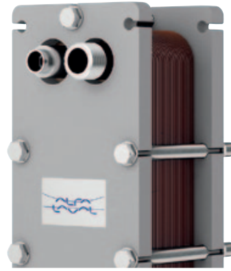
◀ CB60 , copper brazed plate heat exchanger. The brazing material seals and holds the plates together at the contact points ensuring optimal heat transfer efficiency and pressure resistance.
